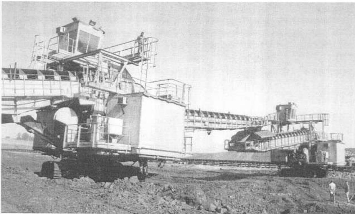
Modern opencast mining machine, In-Pit Coal Crusher in operation at Piparwar OCP
