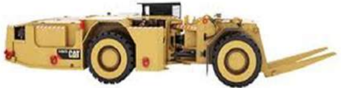
Forklift for squaring of Powered Supports in correct position - upto 60 te
